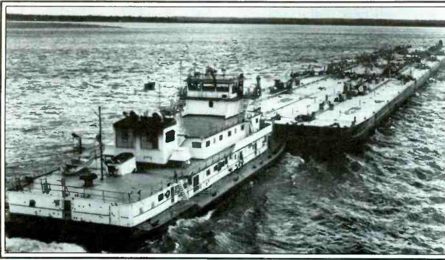
Towboat and petroleum barge moving some 185,000 barrels of petroleum products on the Mississippi River south of Memphis, Tennessee. RTTY monitors will be seeing more and more U.S. merchant marine vessels using RTTY communications in the future. (Photo courtesy of The American Waterways Operators, Inc.)
