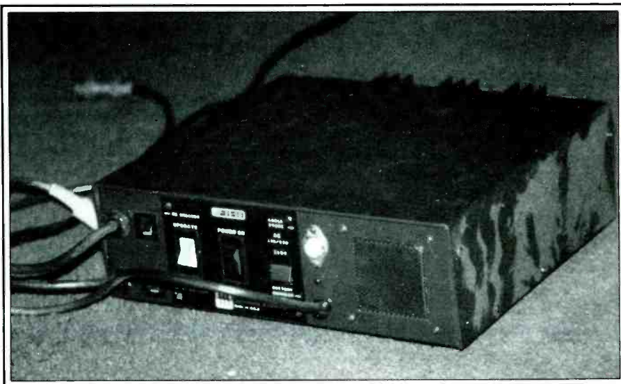
The 110-volt power pack for the MP-25.
